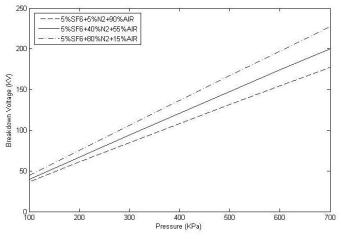
Fig. 12. Effect of gas pressure on the breakdown voltage for various fractonal concentrations of  $SF_6$ - $N_2$ -Air gas mixtures.
