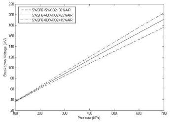
Fig. 11. Effect of gas pressure on the breakdown voltage for various fractonal concentrations of SF<sub>6</sub>-CO<sub>2</sub>-Air gas mixtures.
