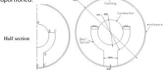
Fig. 3. Gas insulated bus duct with disc-spacer of epoxy material
