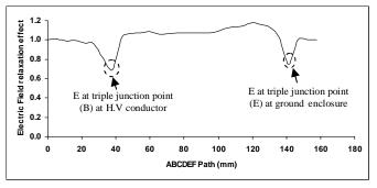
Fig. 6. Electric field relaxation effect ( $E_{FGM}$  /  $E_{uniform}$ ) by introduction of the U-shape FGM spacer.
