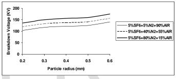
Fig. 15. Effect of particle radius on the breakdown voltage for various fractional concentration of  $SF_6$ -N<sub>2</sub>-Air mixtures.
