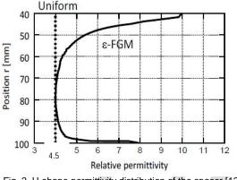
Fig. 2. U-shape permittivity distribution of the spacer [12].
